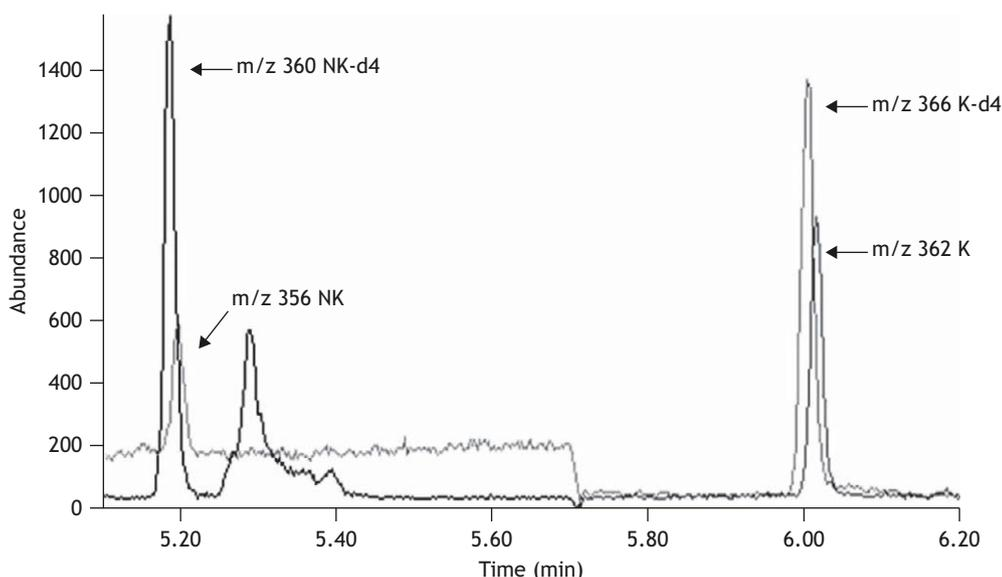
**Figure 2** Gas chromatography-mass spectrometry (selected ion monitoring mode) chromatogram of a neonatal hair sample with ketamine (K) and norketamine (NK), and K-d4 and NK-d4 as internal standards.
