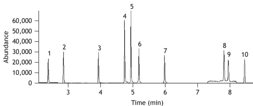
**Figure 1** Gas chromatography-mass spectrometry (selected ion monitoring mode) chromatogram of samples spiked with 5 ng/mg of the target drugs after derivatization with heptafluorobutyric acid anhydride. 1=amphetamine; 2=methamphetamine; 3=3,4-methylenedioxyamphetamine; 4=3,4-methylenedioxy methamphetamine; 5=3,4-methylenedioxyethylamphetamine; 6=norketamine; 7=ketamine; 8=morphine; 9=codeine; 10=6-acetylmorphine.
